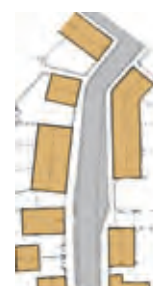
Plot vehicle tracking path, to check carriageway width is sufficient
